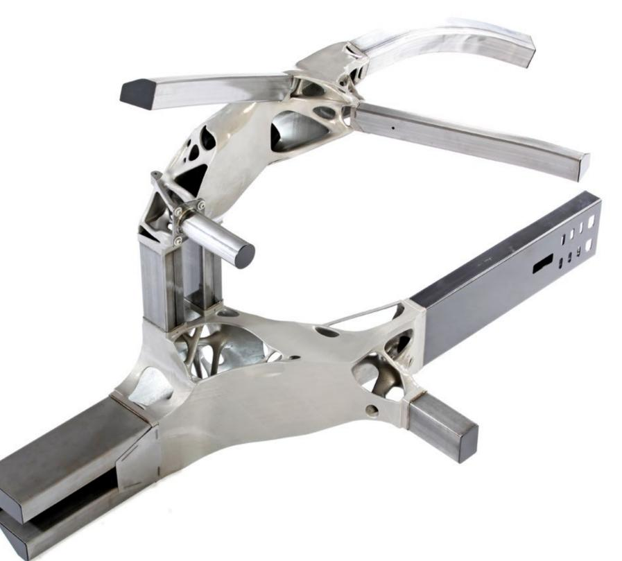
The laser cutting process was used to cut profiles in such a way that it ensured controlled deformation in case of a crash, thus making the car safe to drive.
